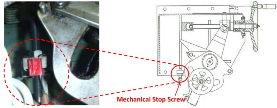
Mechanical stop screw sealed by wire
