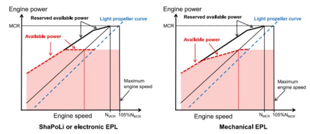
Figure 1: Engine load diagram on Shaft/Engine Power Limitation
