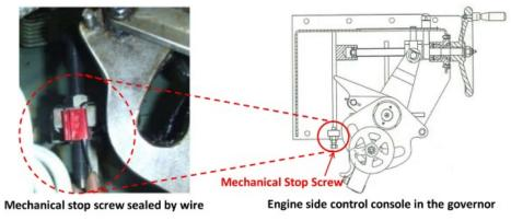
Figure 2: Sealing of mechanical stop screw
