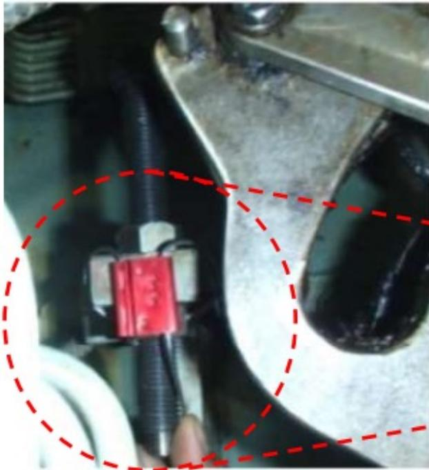
Mechanical stop screw sealed by wire
