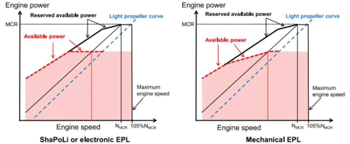
Figure 1: Engine load diagram on Shaft/Engine Power Limitation
