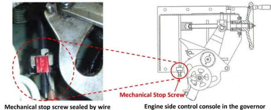
Figure 2: Sealing of mechanical stop screw
